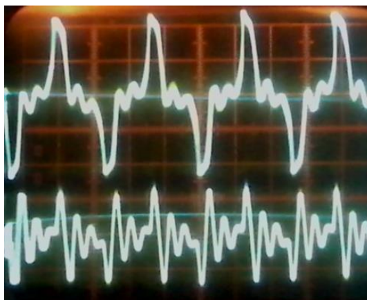
Figure 6. Oscillograms of voltage and current changes in the discharge circuit when supplied with pulsed voltage
