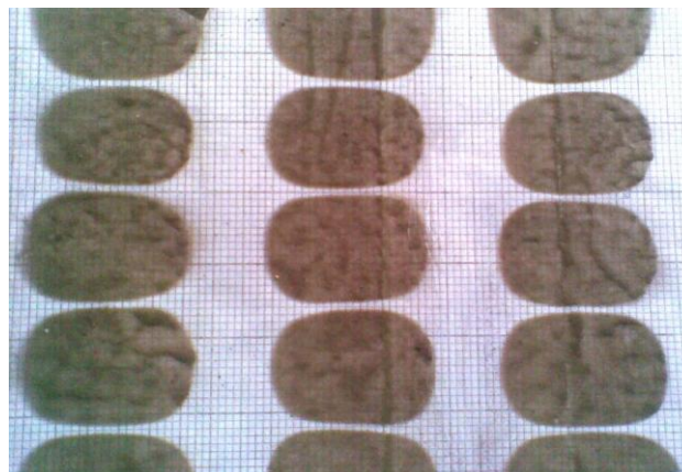
Figure 8. Pattern of spots of deposited dust from corona needles 20 mm long, with their in-line arrangement and the distance between the needles in the rows is twice as large as the distance between the needles in the rows (cells on a substrate 2x2 mm)
