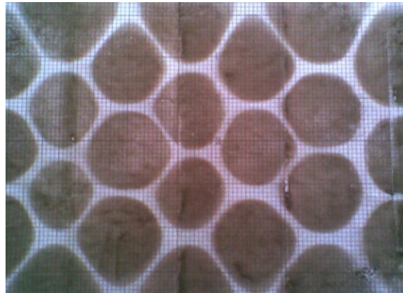
Figure 7. Pattern of spots of deposited dust from corona needles 25 mm long, with their staggered arrangement and the same distance between the needles in the rows and between the rows of needles
