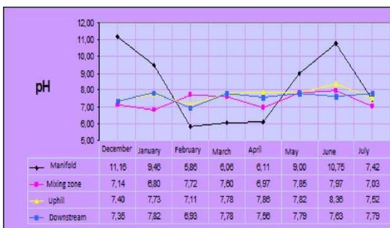
Figure 3: Monthly change in the pH of the wastewater
