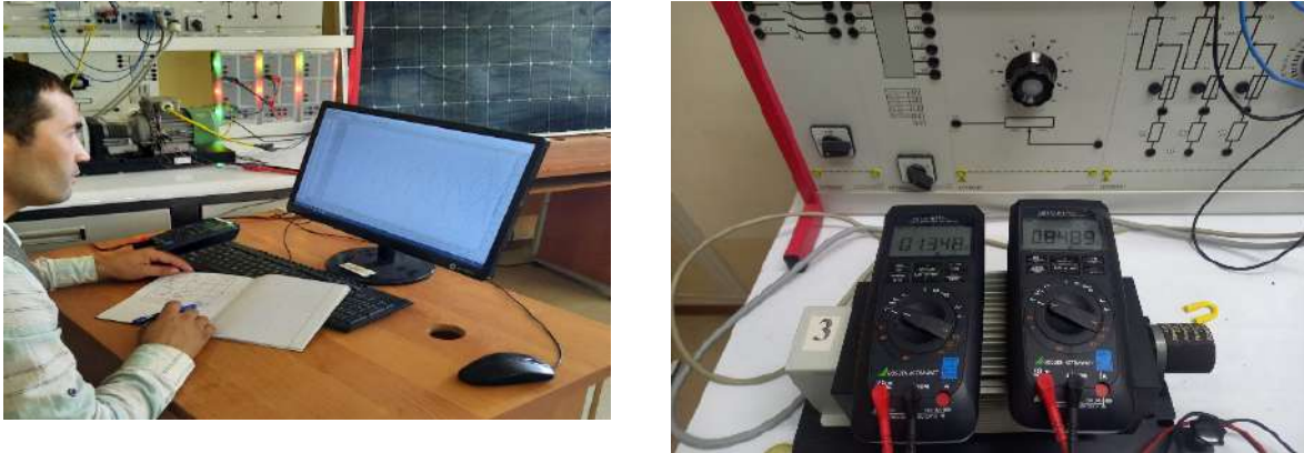
Fig. 3. The process of receiving a signal from an asynchronous motor and its measuring circuit provided by the energy source produced by solar panels in CAYSLAB laboratory devices
