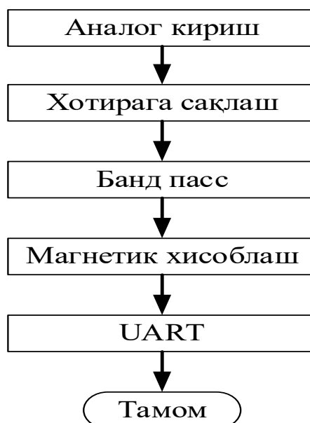
2.9-rasm. Demulator blok diagrammasi
