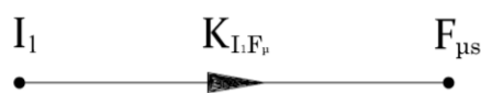
2.2-rasm. I_1 stator tokini F_{\mu s} magnit yurituvchi kuchga aylanish jarayoni modeli.
