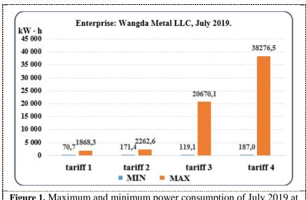
**Figure 1.** Maximum and minimum power consumption of July 2019 at Wangda Metal LLC
