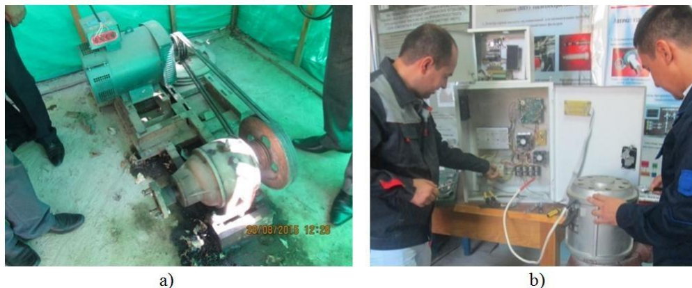
Figure 4. Place of installation of the generator and reducer of the device (a) and the process of preparation of the generator and power unit for operation (b)
