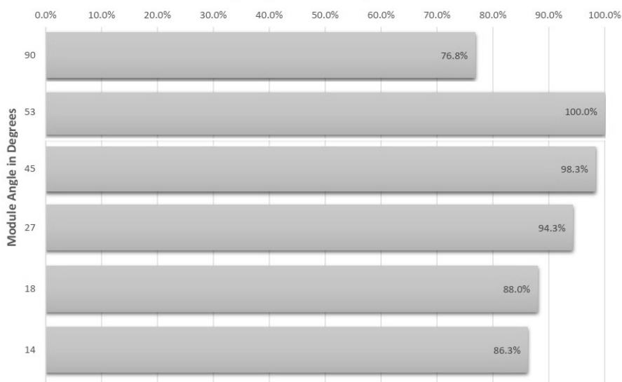
Fig. 5. The efficiency of electricity production compared to the installation of solar panels at different angles
