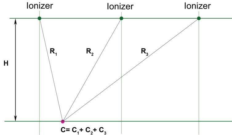
**FIG. 7:** The scheme for calculating ion concentrations:  $H$ , height from the calculated point to the line of location of the ionizers;  $R_i$ , the distance from the calculated point to the corresponding ionizer
