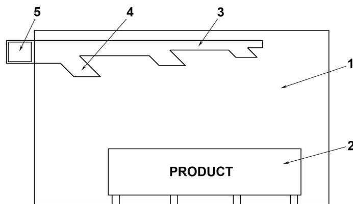
**FIG. 3:** The arrangement of ionizers in the fruit storage: 1) storage room; 2) stored product; 3) air duct; 4) air duct vents where ionizers are installed; 5) power supply for ionizers
