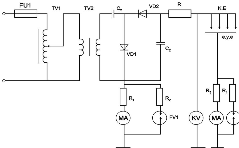
**FIG. 1:** Schematic diagram of the air ionizer: KE) discharge electrodes; e.y.e) grounded electrode; R) voltage divider; TV2) step-up transformer; TV1) autotransformer; FV) dischargers; mA — milliammeters, and kV — kilovoltmeter
