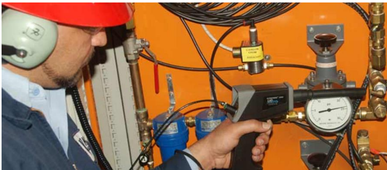
24 rasm. Havo bosimini o'lchash.
