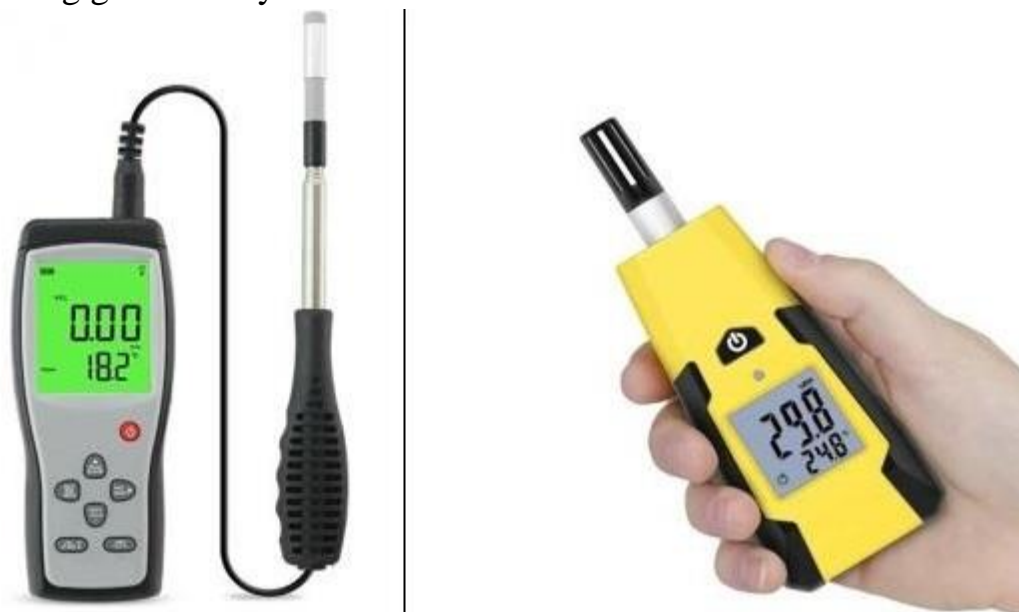
26 rasm. Termometr va anemometr yordamida o'lchash.
