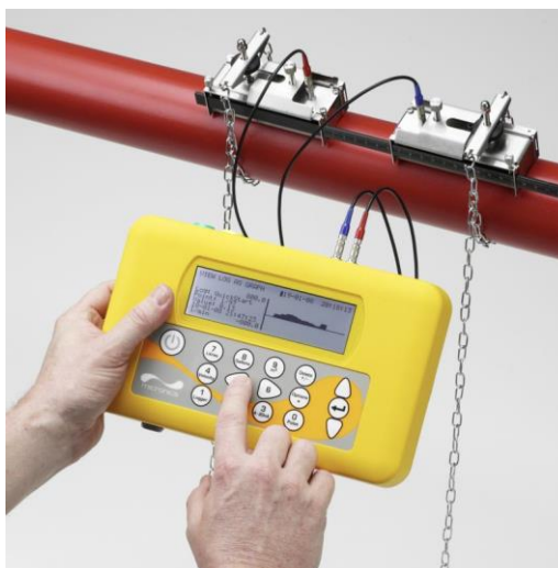
5 rasm. Ultratovushli suyuqlik oqim o'lchagichi Portaflow 330 A + B.
