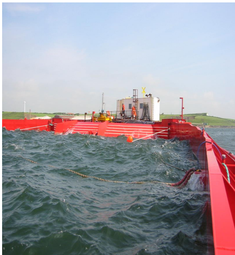
Wave Dragon Overtopping Device, Denmark 1.5 to 12 MW of capacity
