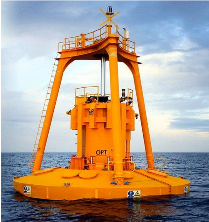
PB150 PowerBuoy with peak-rated power output of 150 kW. USA
