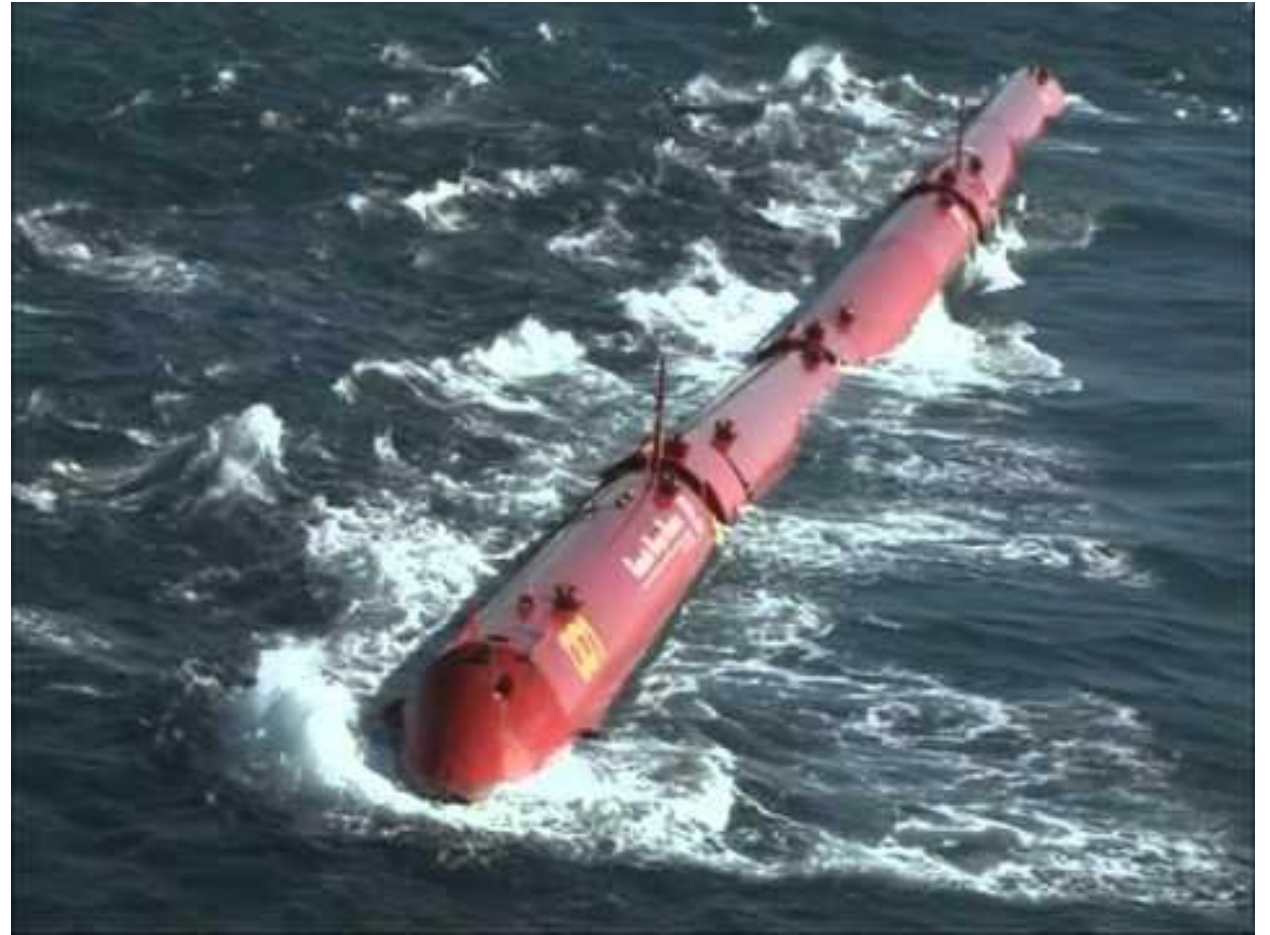
750 kW Pelamis Wave Energy Converter, Scotland
