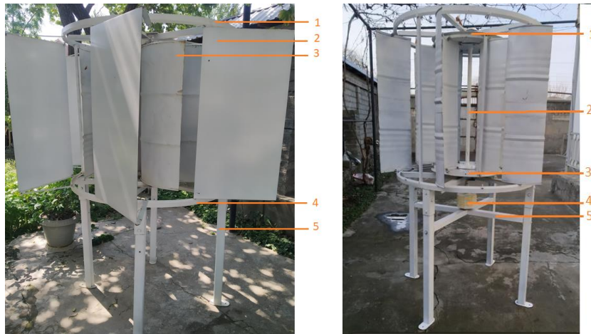
Fig. 4. Wind power plant. 1,4 - rings that hold the guide wings; 2 - guide bars; 3 - working wheel blades; 5 - holding legs; 6,7 - discs holding the main wings; 8 - generator; 9 - frame holding the generator; 10 - shaft
