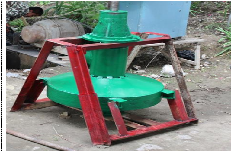
Figure 5. Prototype of a reactive micro-hydroelectric power station
