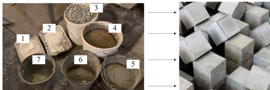
Figure 1. Type of materials and manufactured samples: 1, 2 – concrete modifier "Embelit"; 3 – crushed stone; 4 – washed sand; 5, 6 – Portland cement; 7 – drinking water with plasticizer
