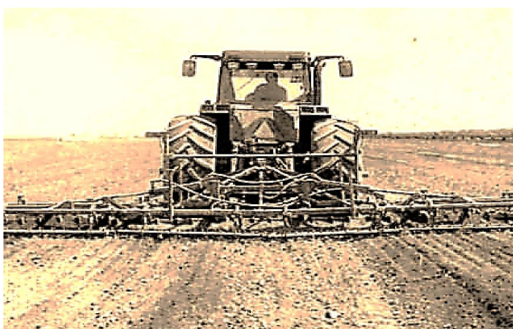
Figure 3. Pre-sowing leveller TEA-7 in aggregate with Magnum 8940 tractor in operation (rear view).
