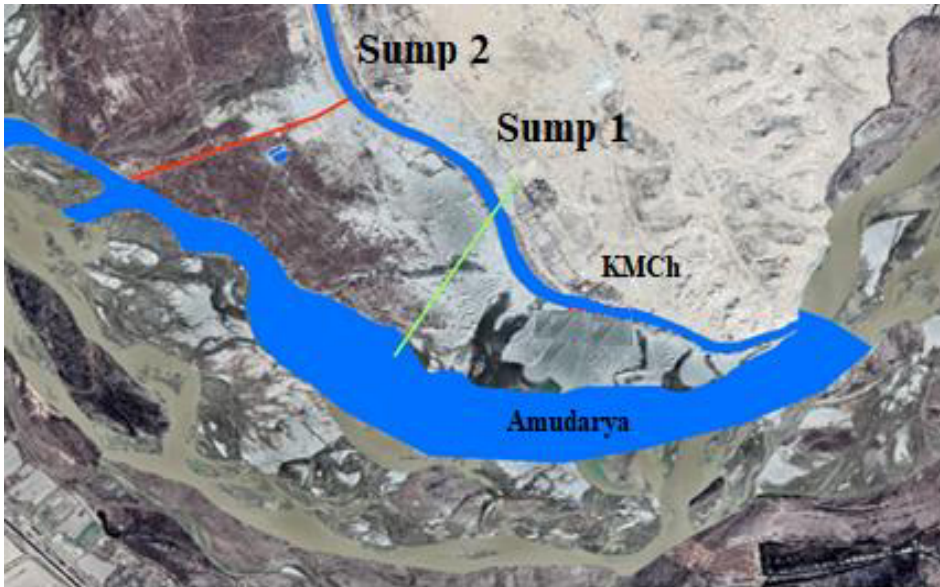
Fig. 5. Space view of the location of the proposed sediment basin on the Karshi Main Channel
