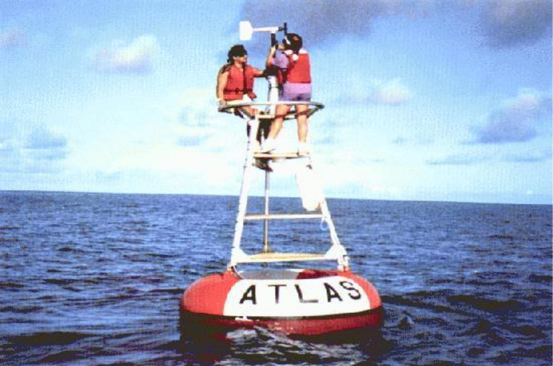
Servicing an ATLAS mooring of the TOGA-TAO Array. ATLAS moorings measure surface winds, air temperature, relative humidity, sea surface temperature, and subsurface temperature to depths of 500 m.
