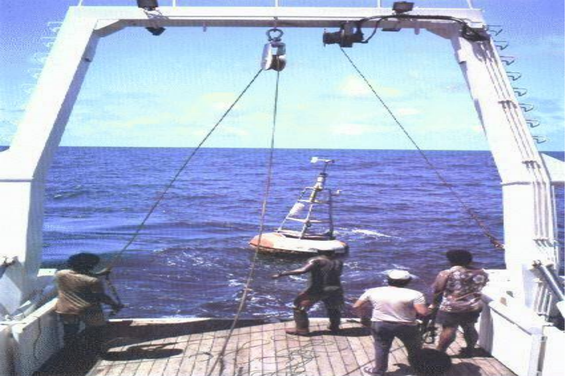
Recovering an ATLAS mooring from the French R/V LE NOROIT in the western equatorial Pacific Ocean. A total of 59 ATLAS moorings are deployed at present in the equatorial Pacific as part of the TOGA-TAO Array.
