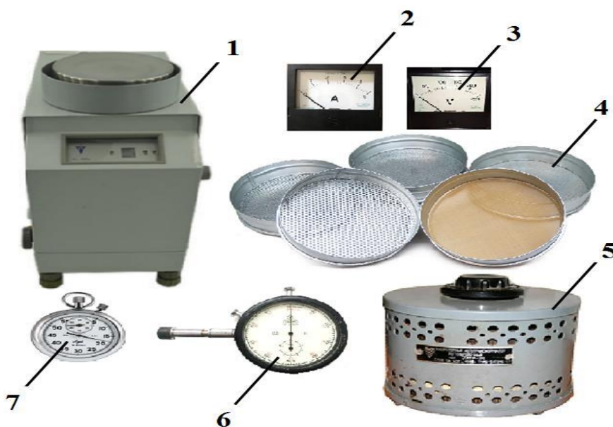
1-VLKT-500 analitik tarozi; 2- M 381T42 ampermetr; 3- M 381 voltmetr; elaklar; 5- LATR-1M avtotransformator; 6- TCH10-R taxometr; 7- Agat 4295V sekundomer.
