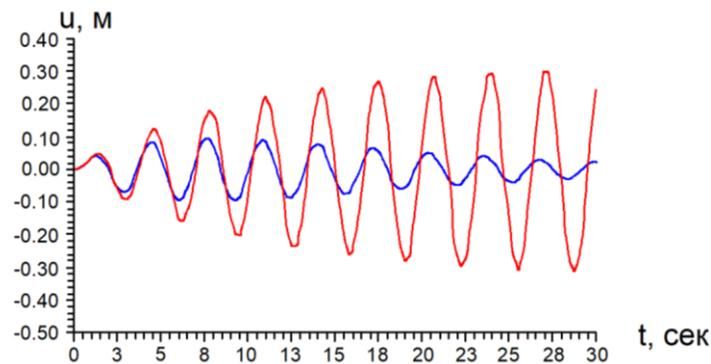
**FIGURE 5.** Forced vibrations of the point  $z = 325\text{m}$  of the beams, taking into account the nonlinear viscoelastic properties of the material under the impact  $\ddot{W}_0 = 0.1A\sin(1.68t)\exp(-0,1t)$ : ——— - nonlinear-viscoelastic solution; ——— - linear-elastic solution.
