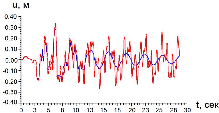
**FIGURE 3.** Forced vibrations of the point ( $z = 325\text{m}$ ) of the beams under the effect of the accelerogram of the Gazli earthquake: ———— - viscoelastic solution;
