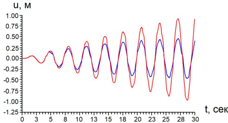
**FIGURE 1.** Forced vibrations of the point  $z = 325m$  of the beams at resonance mode  $\ddot{w}_0 = 0.1A \sin(1.68t)$ : — blue — viscoelastic solution; — red — elastic solution.
