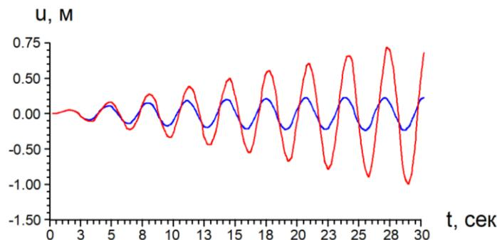
**FIGURE 4.** Forced vibrations of the point  $z = 325m$  of the beams taking into account the nonlinear viscoelastic properties of the material under the impact  $\ddot{W}_0 = 0.1A\sin(1.68t)$ : ——— - nonlinear-viscoelastic solution; ——— - linear-elastic solution.
