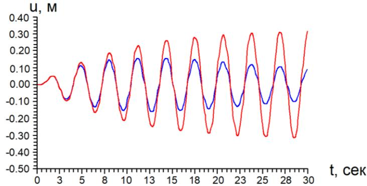
**FIGURE 2.** Forced vibrations of a point ( $z = 325\text{m}$ ) of beams under the impact  $\ddot{w}_0 = 0.1A \sin(1.68t) \exp(-0.1t)$ :
