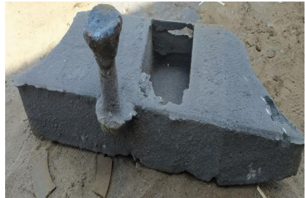
Pic. 4. Defects observed in the sand – clay molding of the lifting roof detail.
