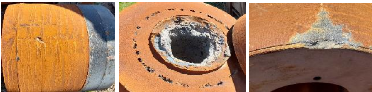
Pic. 1. Effect of non – metallic inclusions and porosity on alloy quality (after machining)
