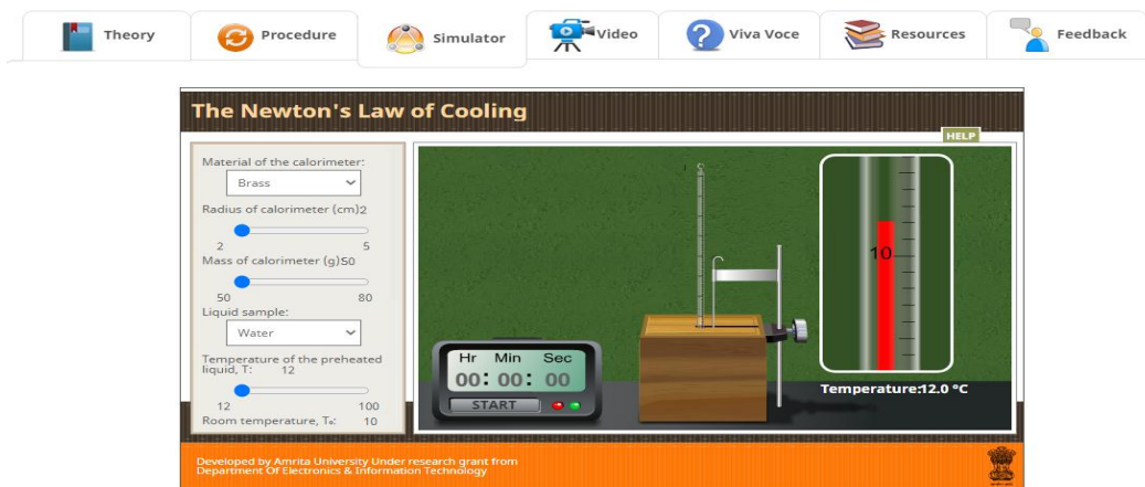
1-picture. Study of Newton's cooling law using a virtual laboratory with the Vernier digital laboratory
