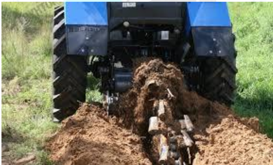
2-rasm. ETS-165 rusumli transheya qazuvchi mexanizmning ish jarayoni.
