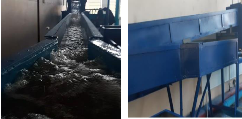
Fig. 6. Side outlet water well model.
