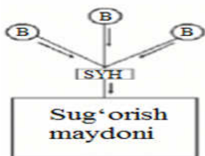
5-rasm. Buloq manba-laridan sug'orishda foydalanish sxemasi
