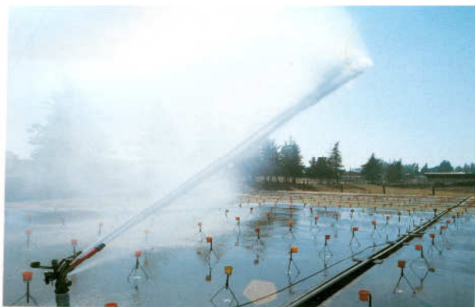
34-rasm. Yomg'ir latib sug'orishda suv sarflarini aniqlash
