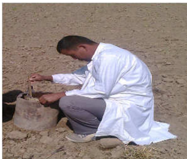
14-rasm. Tuproqning suv o'tkazuvchanligini dala sharoitida aniqlash.
