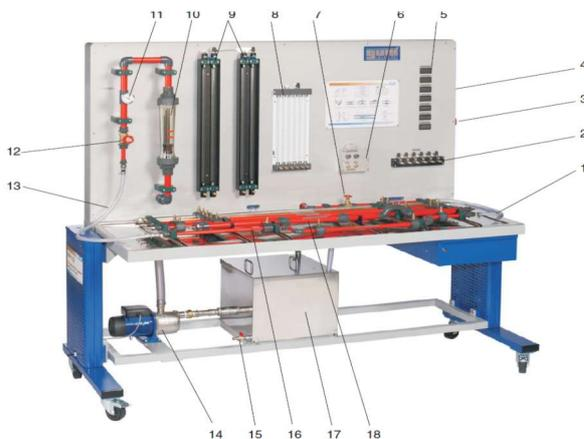
**Fig.1.** Exterior view of the experimental unit G.U.N.T. HM 112: 1. Return hose; 2. Electronic pressure switch; 3. Main Eraser; 4. Pump switch (concealed); 5. Digital pressure display; 6. Differential pressure reducer; 7. Check valve; 8. Six-pipe pressure gauge; 9. Two-pipe pressure gauge; 10. Flowmeter-Rotameter; 11. Thermometer; 12. Pressure reducing valve; 13. Inlet hose; 14. Pump; 15. Drain valve; 16. Different units of measure; 17. Water tank; 18. Interchangeable measuring objects
