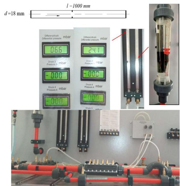
**Fig. 3.** Natural and electronic pressure readings in the copper pipe
