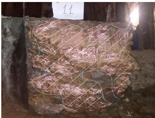
Fig 5. Shear surface after testing dies No. 11.
