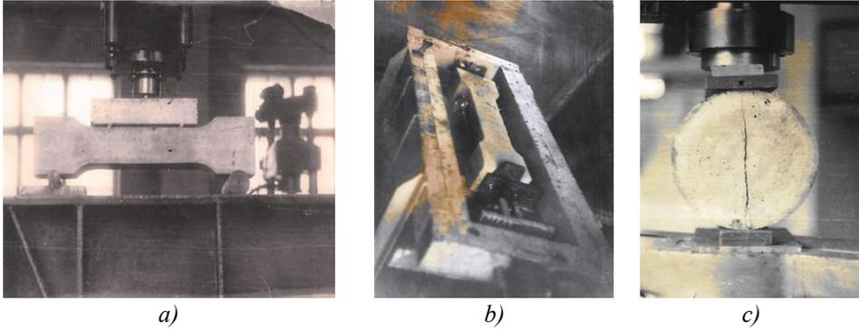
**Fig.2.** General view of the test specimens to obtain the crack resistance characteristics of concrete in four-point bending (a), stretching (b), and cracking (c).
