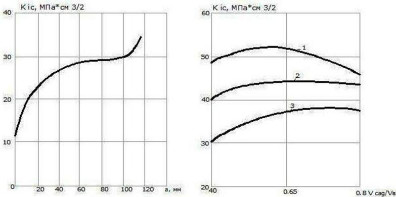
**Fig.4.** Dependence of KIC on notch length and expanded clay content: 1- bending, 2- stretching, 3- cracking.
