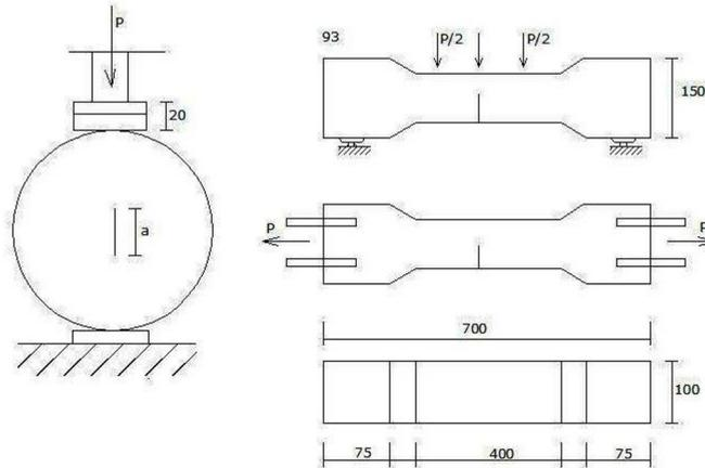
**Fig 1.** Scheme of testing prototypes (splitting, four-point bending, and tension of beam samples with various artificial notches).
