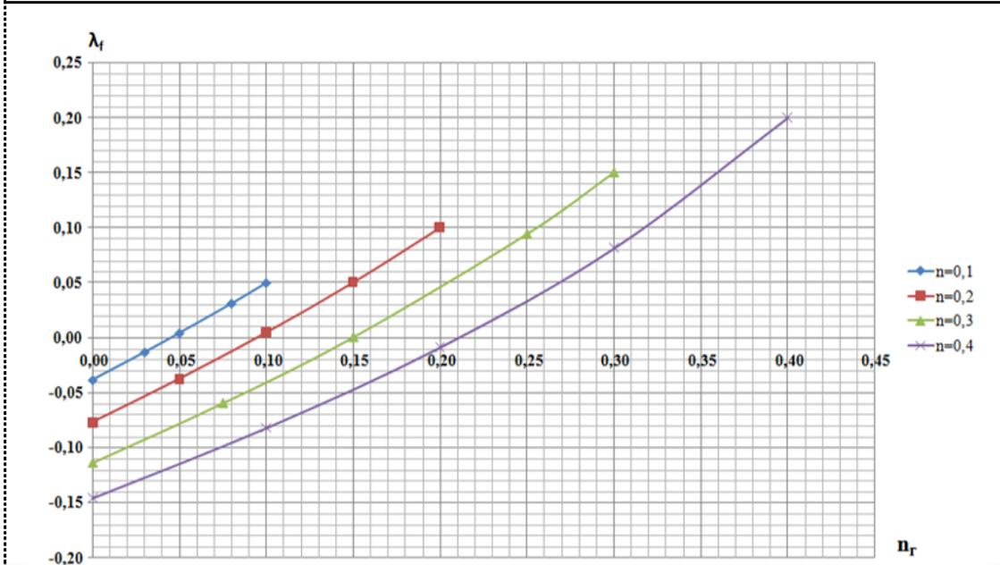
**Figure 3.** Impact of contraction degree of combined dam on dynamic axes of flow
