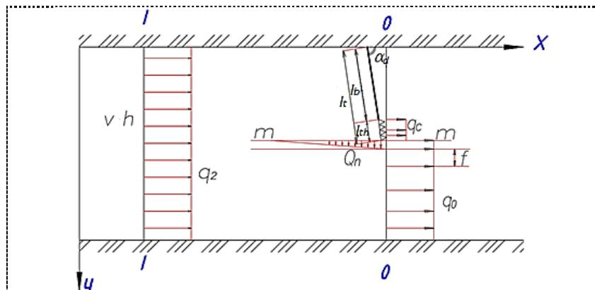
**Figure 1.** Scheme of deflection of the dynamic axes of flow unilaterally contracted by a combined dam.
