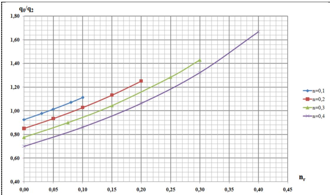
**Figure 2.** Impact of contraction degree of combined dam on relative specific discharges in contracted section
