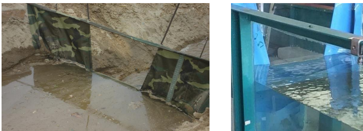
Figure 1. Testing the portable water measuring weir in field and in laboratory.
