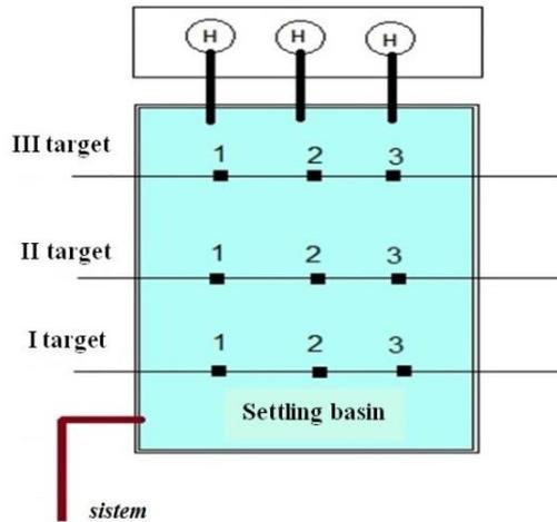
**Fig. 2.** Drip irrigation system of "Islam" farm. The scheme of sampling of mud in the Settling basin.
