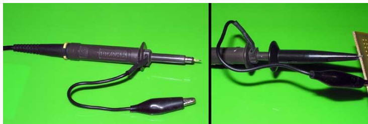
2.6-rasm. Zamonaviy Ossillografning shchupi, chapda "ignali", o'ng tomonda qismali
