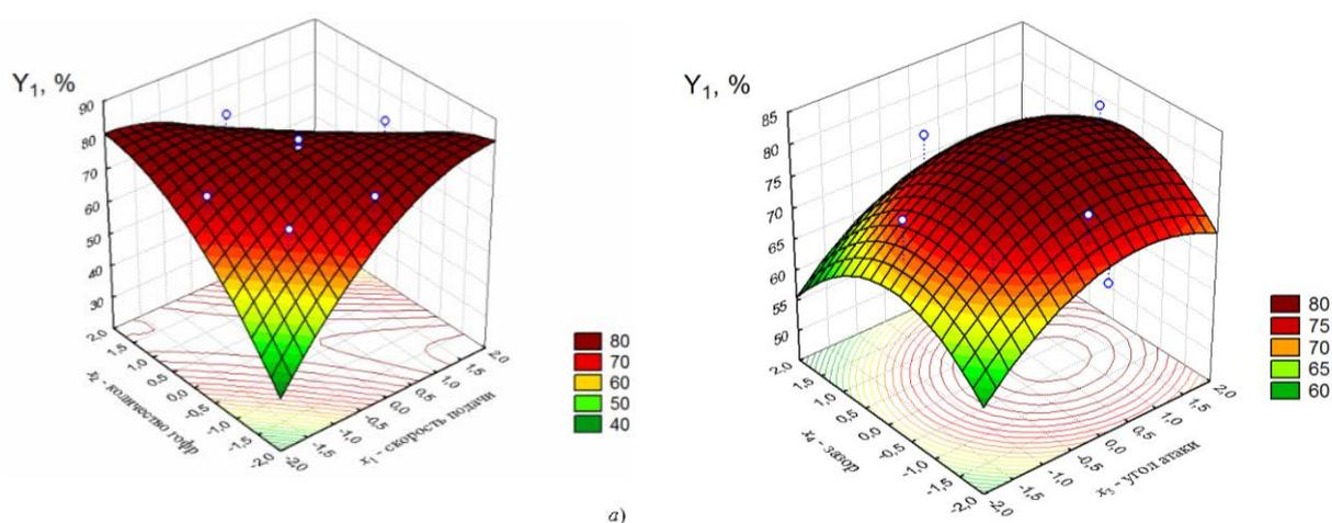
**Figure 5.** Response and contour of threshing grain of dry short-stalked wheat
