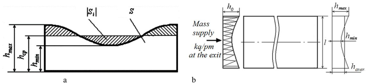
**Figure 2.** The initial state of the grain mass (a) and to the transformation of the mass across the width of the thresher of the combine harvester (b)
