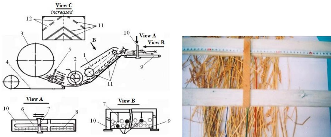
**Figure 4.** The technological scheme of the device with the bread mass of dry short-stemmed: 1- conveyor; 2-auger; 3 reel; 4-conveyor feeder; 5-U-shaped measuring frame; 6-slot frame; 7-clamp 8-meter ruler; 9-discharge conveyor; 10-frame; 11-corrugation device; 12 - discreteness of the corrugation
