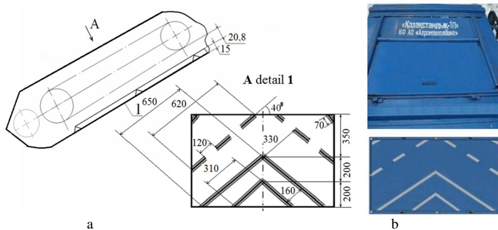
Figure 6. Structural-technological scheme (a) and experimental sample of an inclined chamber with device (b)
