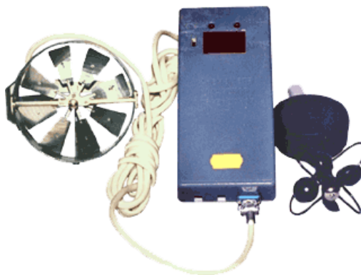
1.1-rasm. АП1-1 rusumli tsifrali ko'chma anemometrning tuzilishi.
