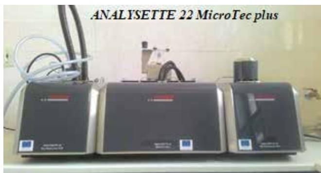
Figure 1. ANALYSETTE 22 MicroTec plus: a unit for determining the unit of measurement for dry and wet samples using a laser
