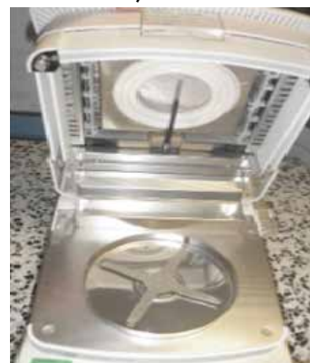
Figure 2. SARTORIUS MA 150: Moisture measuring device
