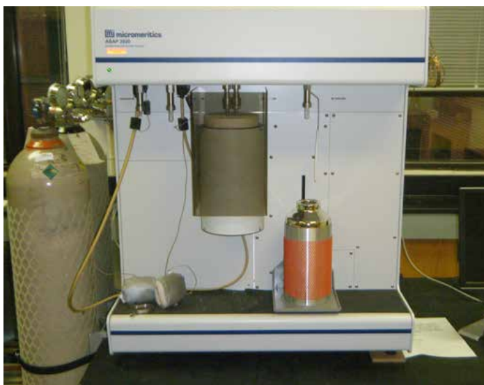
Figure 4. ASAP 2020 Micromeritics: a device for studying the nano-porous structure of hydrolytic lignin
