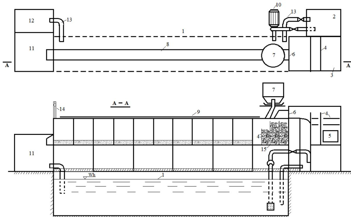
**Figure 1.** Scheme of a flat glazed experimental unit: 1-main pool; 2-main tank; 3-water intake tank; 4-dampener grids; 5-connecting pipe; 6-spillway; 7-dispenser; 8-tray; 9-rail; 10-centrifugal pump; 11,12-sump pool; 13-return pipes; 14-control panel; 15-chips-dampers.
