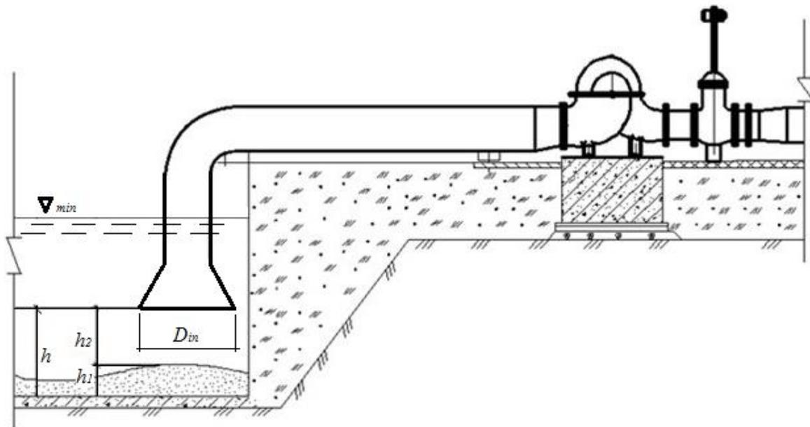
**Figure 8.** The proposed scheme for determining the height of the pumping unit suction pipe inlet relative to the riverbed bottom.
