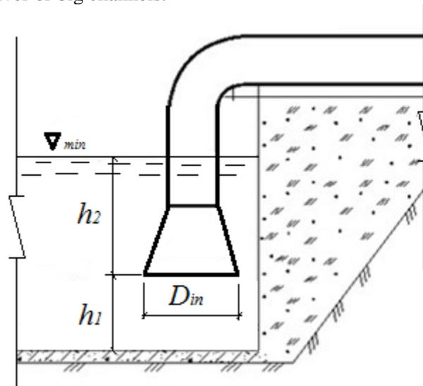
**Figure 7.** Existing scheme for determining the height of the inlet of a vertically installed suction pipe of the pumping unit.
