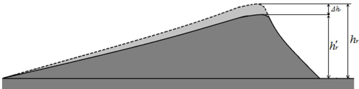
**Figure 6.** Calculation scheme for determining the estimated ridge height.
