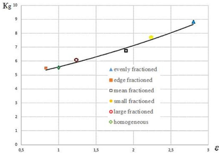
Figure 4. Dependence graph of the coefficient  $K_g$  on the heterogeneity of sediment.
