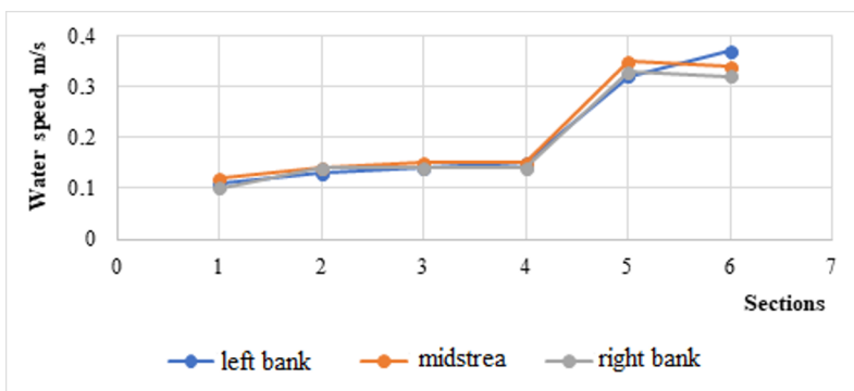
Fig. 8. Flow velocities for the case when the shutter opening height a = 8 \text{ cm} with a channel slope i = 0.02
