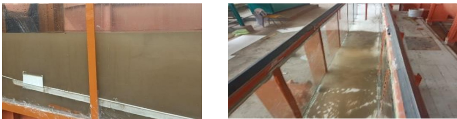
Fig. 7. The process of sedimentation of turbid particles to the bottom of the tray when the water flow reaches the backwater level
