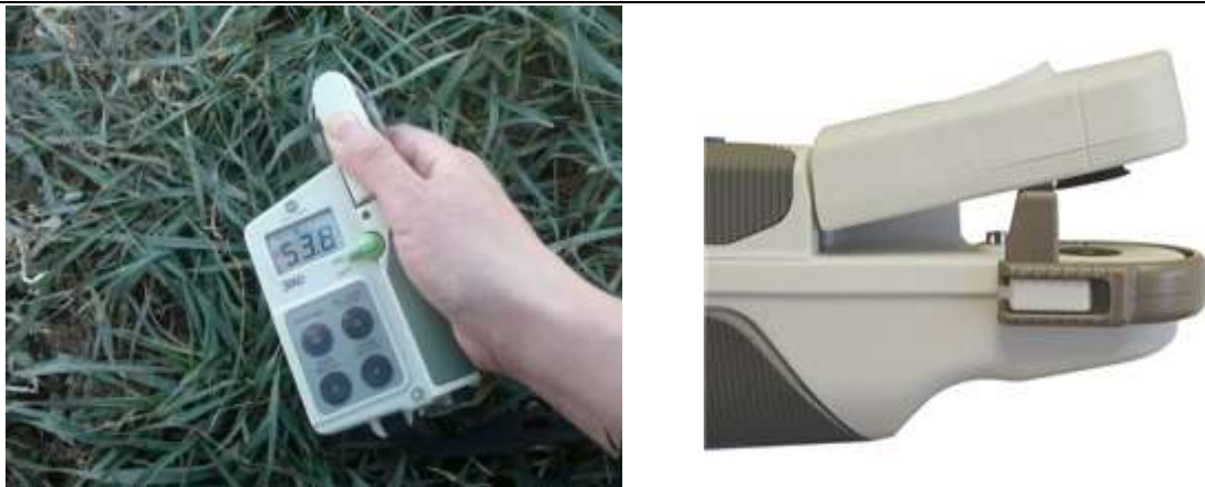
Figure 1. Minolta SPAD-502 chlorophyll meter overview (left) and the part where the leaf is inserted and measured (in it)
