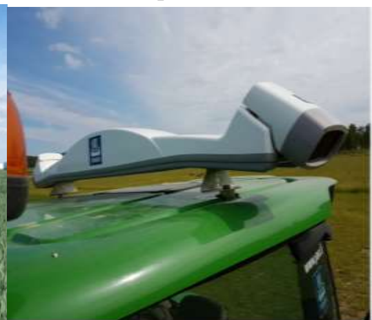
Figure 6. Yara N-Sensor active sensor partitive spark
