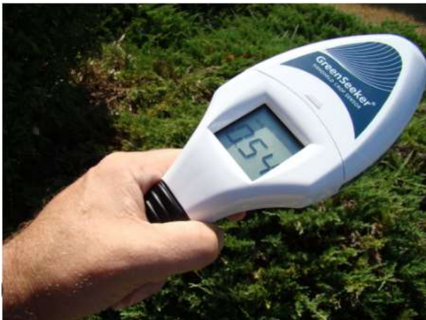
Figure 5. GreenSeeker is a partitive spark that detects plant biomass
