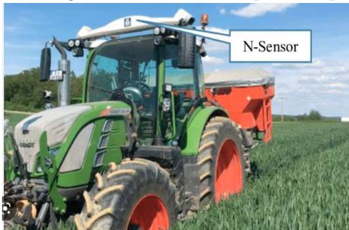
Figure 6. Yara N-Sensor active sensor partitive spark
