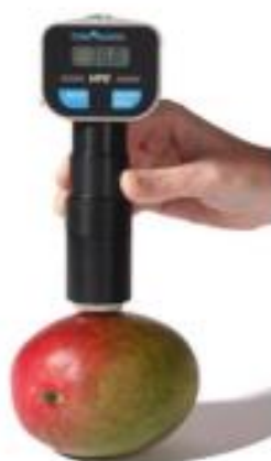
2-rasm. HPE III Fff asbobining anorning qattiqligini o'lchash jarayoni
