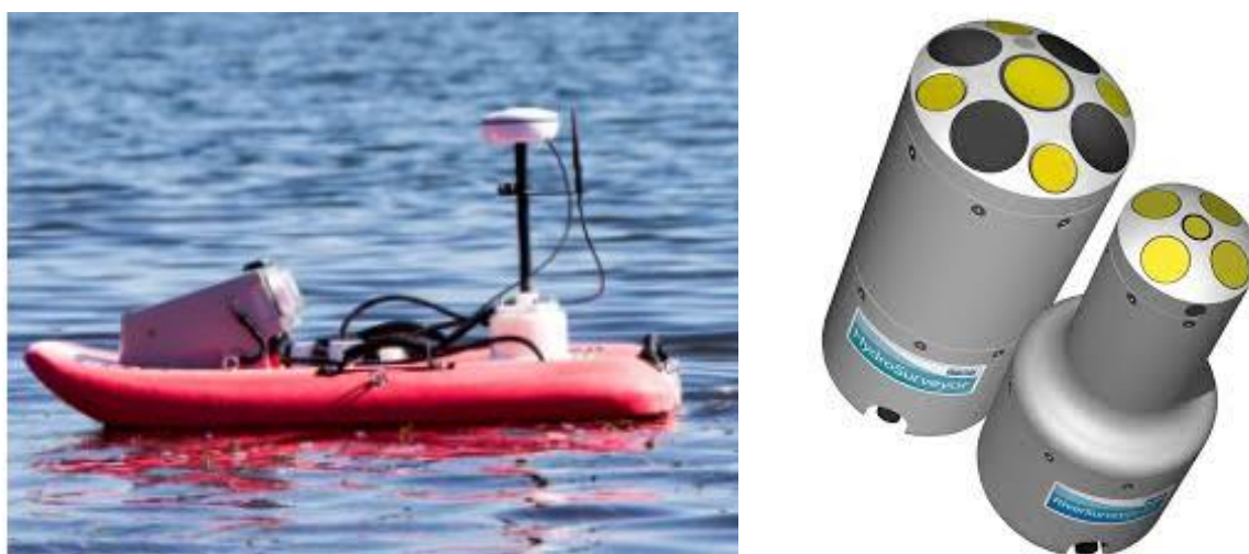
Fig. 1. “SonTekS5” river surveyor Doppler
