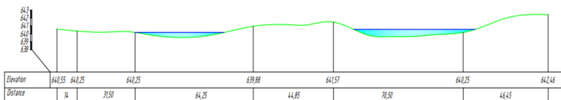
Fig. 3. Cross-section of the Sox stream bed 2019
