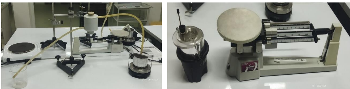
Figure 1. An experimental device for determining the specific heat capacity of solids. "LD Phusica Leafits" (Germany).
