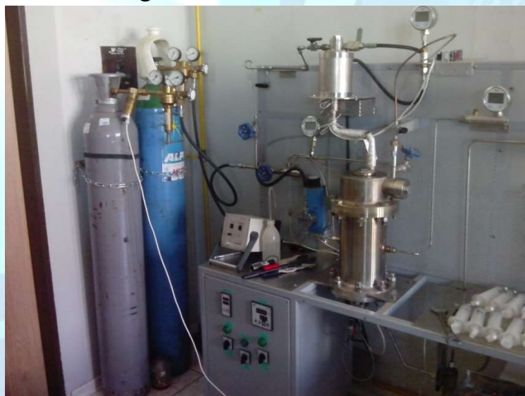
1-rasm. Gaz olish jarayonini o‘rganish uchun laboratoriya qurilmasi[15]
