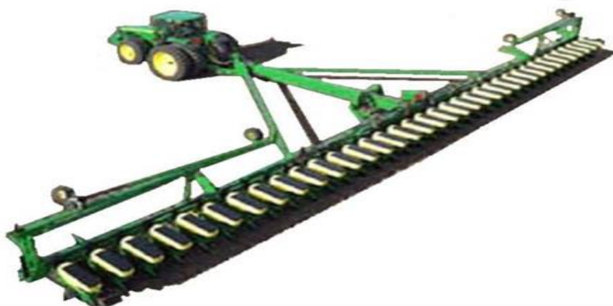
Fig. 8. Trailed thirty-six-row seeder of the “John Deere” company
