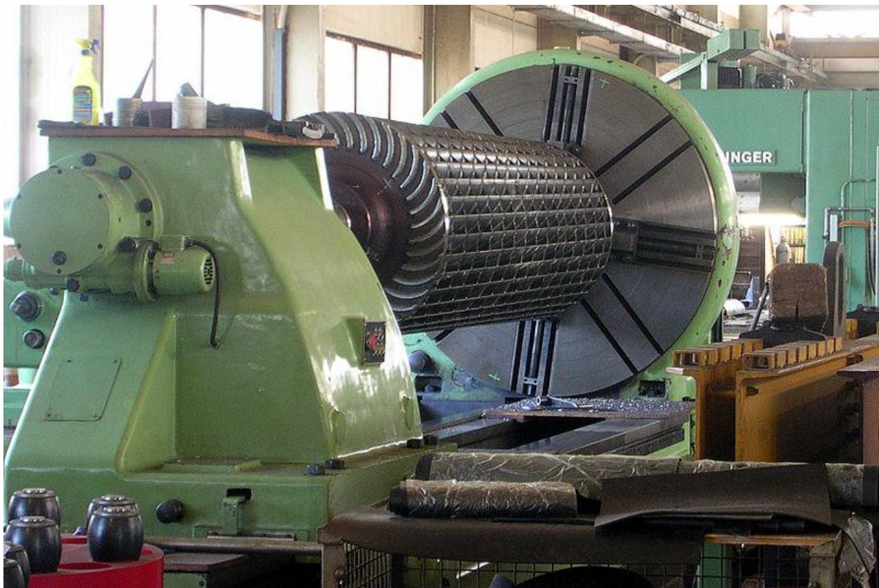
3.9.3-rasm. Ikki karra harakatlanadigan turbinaning rotori
